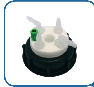
SW60-1-C-4L : 1 entry 1/8", 4 tube fittings and charcoal cartridge emplacement
