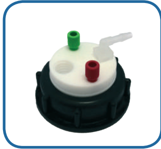
SW60-2-C-1L : 2 entries 1/8", 1 tube fitting and charcoal cartridge emplacement
