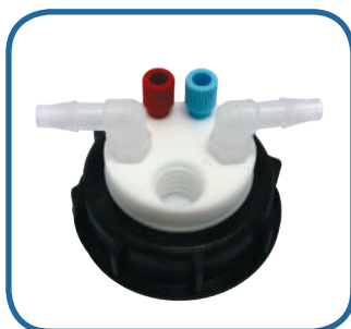
SW55-2-C-1L : 2 entries 1/8", 2 tube fittings and charcoal cartridge emplacement
